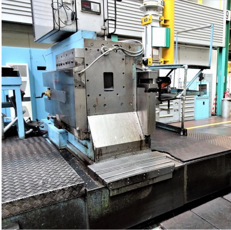
upper carriage with tool holder and work piece measurement
