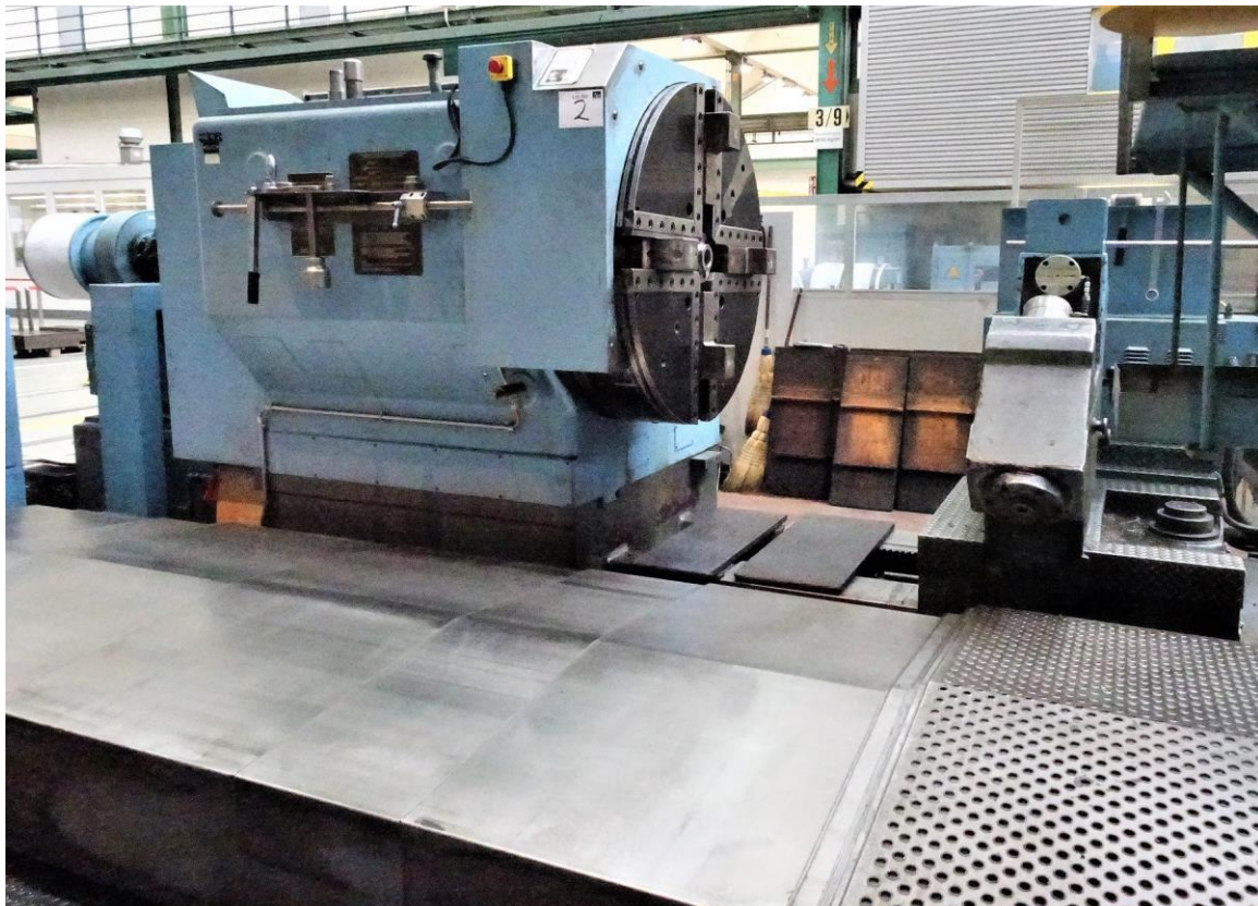
upper carriage with tool holder and work piece measurement
