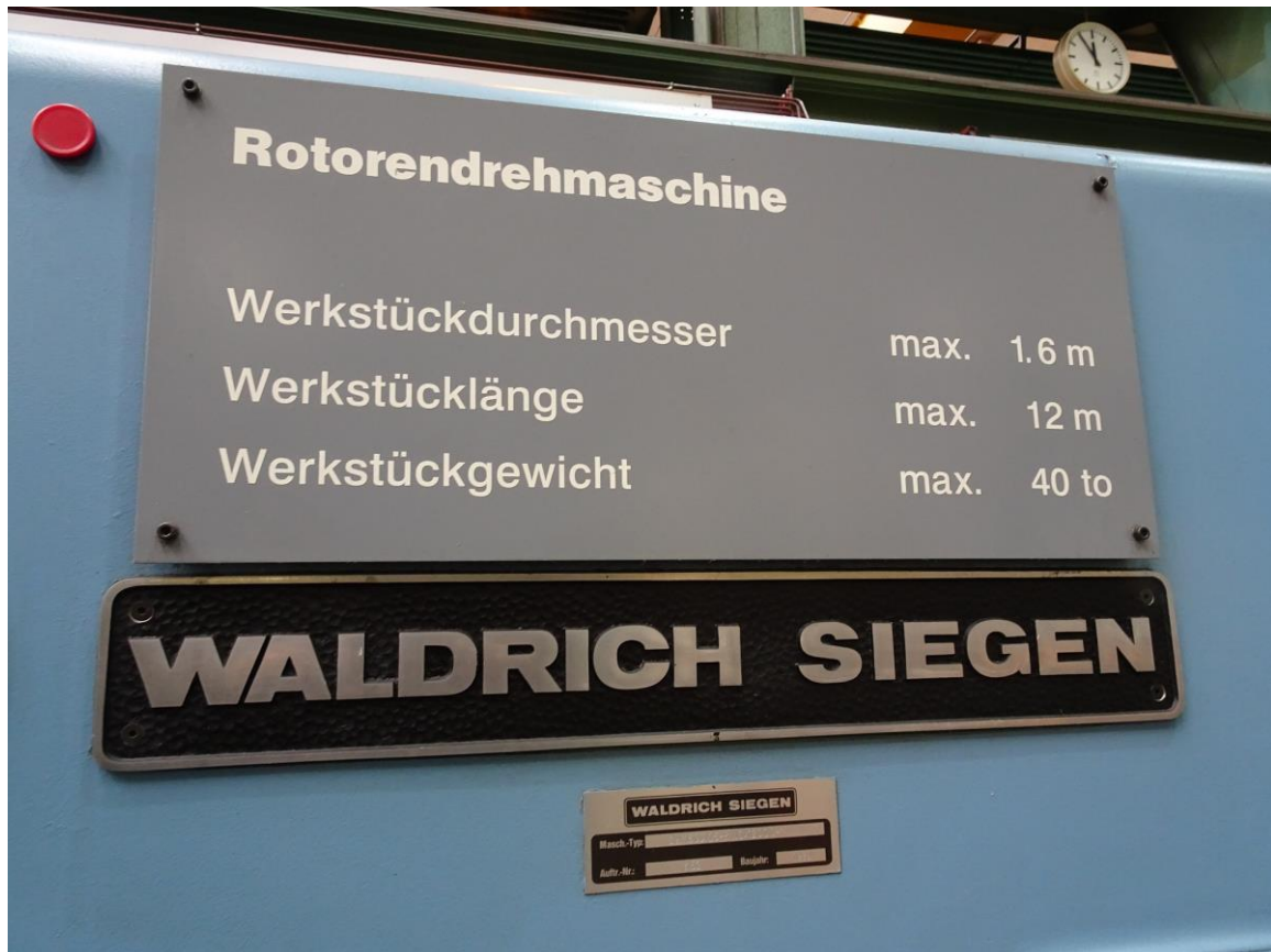
used as turbine rotor finish lathe
