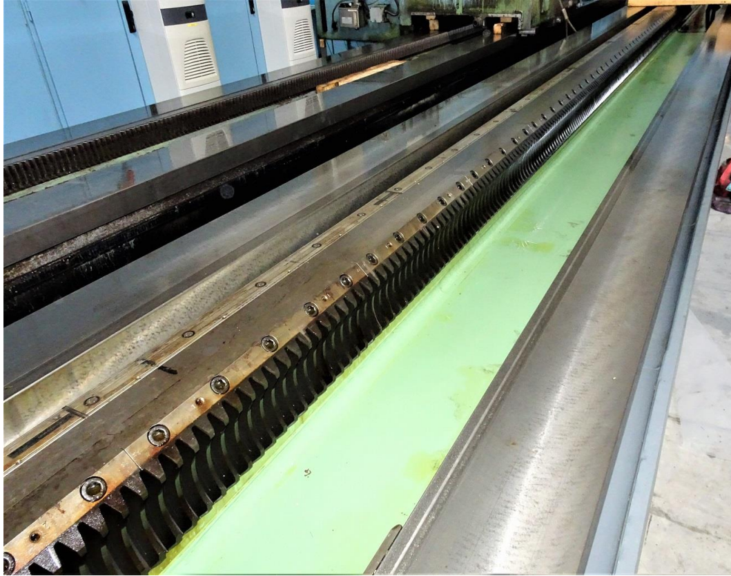
guide ways and hydrostatic worm drive like new
