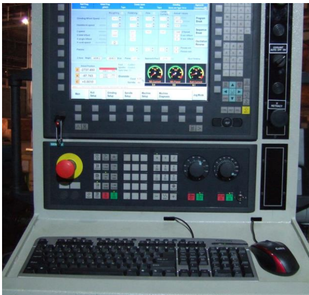
option 2: new CNC control SINUMERIK 840 DsL
